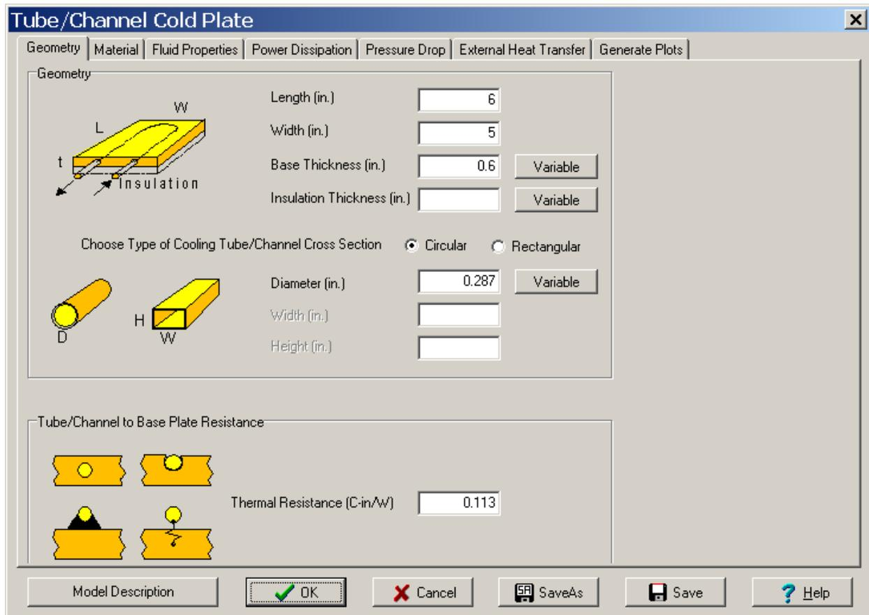
The plate material, 6063-T6 is selected from the material data base on the Material Tab sheet.
