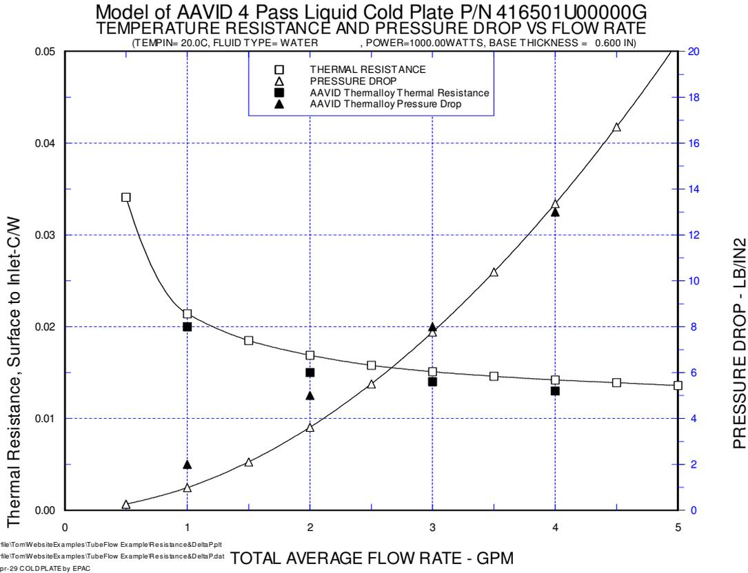
This next section lists the results at the 2.0 GPM flow rate. Note that data was calculated and written out at each of the 10 different flow rates, only the results at 2.0 GPM are shown below.
